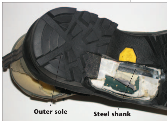
Outersole with embedded steel shank
